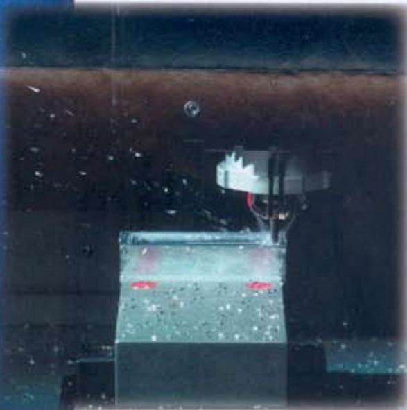
A 1/4" high-speed cutter with 60,000rpm spindle files through a 6061 aluminum sheet.
