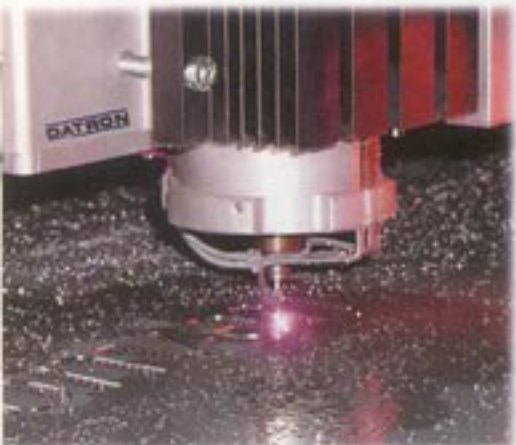
Running at 35,000 rpm with cleanly evaporating alcohol coolant, IntelliCAM avoids the costs of secondary degreasing operations.
