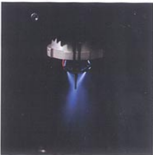
A spindle mounted in the machine spins a microtool with the micro-volume Ethanol coolant spray mist illuminated.
