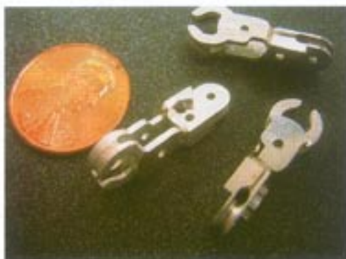
This gripper part demonstrated how EIGERlab's tabletop microfactory is capable of machining, inspecting, assembling and welding.
