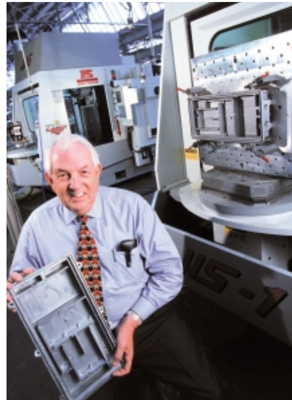
For Jerry Keating, anything that saves time in machining processes also saves money. His investment in HS-1RP HMCs allowed SKS to machine this part in a single setup rather than three, and shave 11 minutes off the production time. The resultant savings of $14 per part on a 12,000 part run netted a tidy $168,000.
