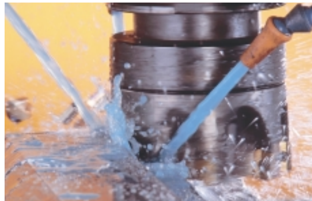
Toughness is the most important criteria for milling because of the interrupted cuts that occur. Milling inserts usually have high cobalt grades that are resistant to thermal cracking, chipping and wear.
