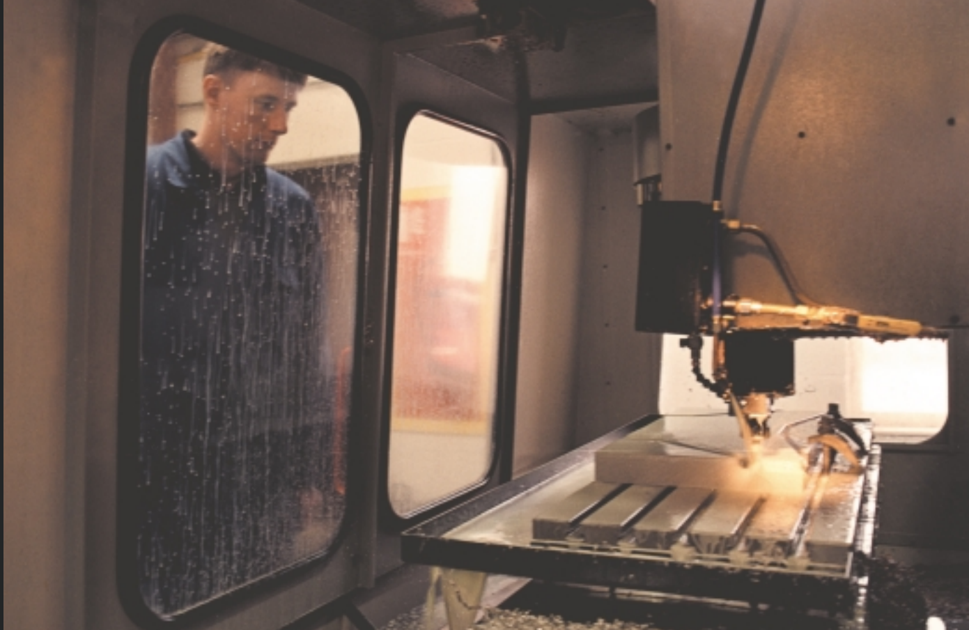
TVR's Paul Howser (programmer/setter) machines a differential carrier plate for the company's Speed Twelve GT race car. The combination of the Haas VF-3 and HyperMill CAD software has allowed TVR to redesign many of their race components to improve strength and reduce weight.
