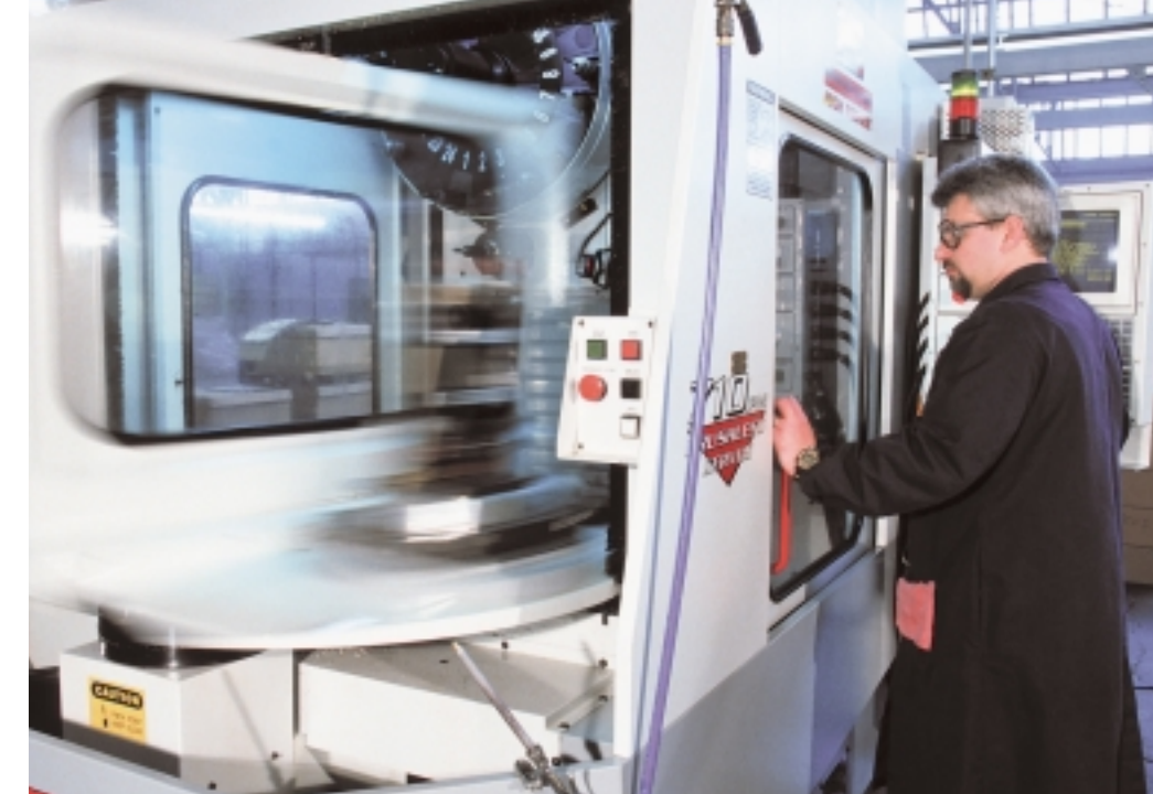
SKS runs their Haas HMCs 20 hours a day in two 10-hour shifts. The built-in pallet changer of the HS-1RP allows programmer/machinist Bruce Thompson, above, to load new material, unload finished parts or setup a new job on one pallet while the other is being machined.
