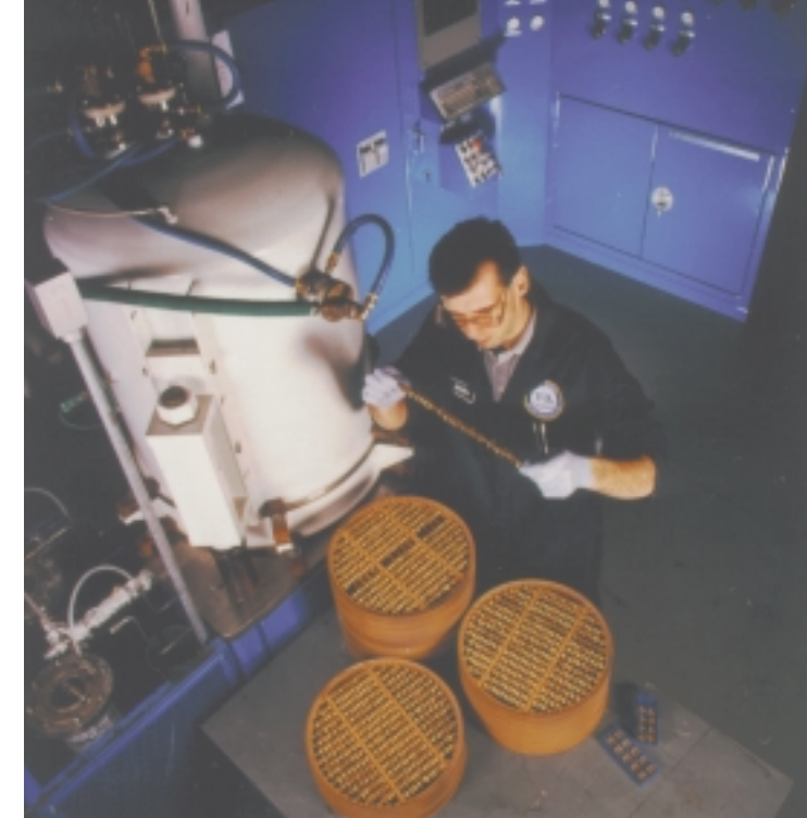
Carbide inserts are loaded into a CVD coating furnace at Valenite Inc., Madison Heights, MI.
