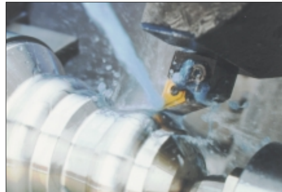
Substrates can be tailored to provide the characteristics necessary for specific applications, such as wear and crater resistance, which are the highest priority for turning inserts.
