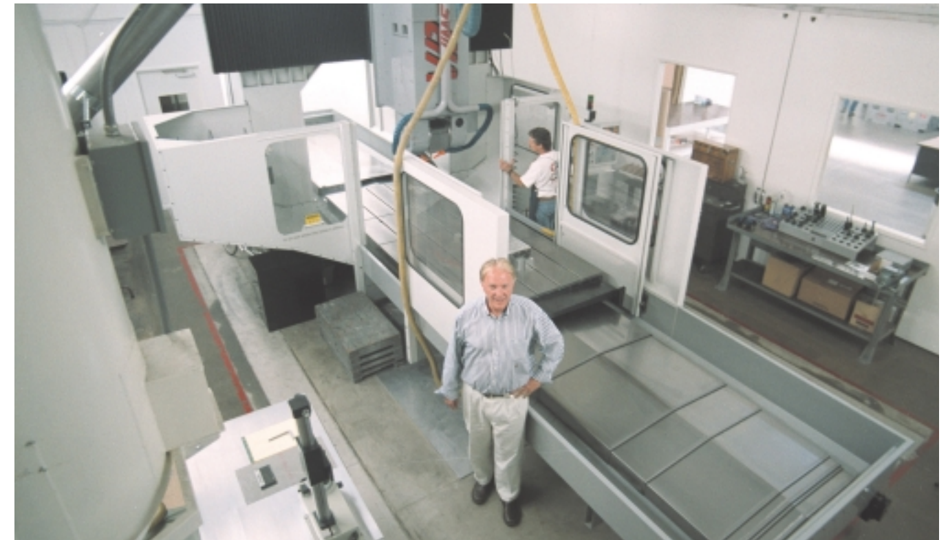
Dan Gurney and the latest weapon in the All American Racers' arsenal, the Haas VB-1 vertical bridge mill. The prototype machine (now in production-Ed) features full 5-axis articulation and travels large enough to machine the molds used for the carbon-fiber body components of the new Eagle 997 CART racer.
