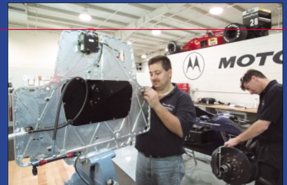
PacWest's build shop, above, is where the CART cars of Mauricio Gugelmin and Mark Blundell are brought to life. Although new cars are received fully assembled from Reynard, PacWest immediately takes them apart and rebuilds them to their own specification.
