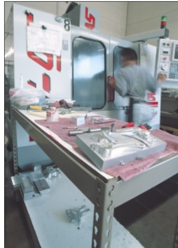
High-tech frame components for GT Bicycles Inc., helped IMD make the change from manual to CNC mills. Here, a Haas VF-0E is used to cut a rear axle bracket for the STS 1000-series bike. With carbon-fiber frames and fully-articulated suspensions, these bikes are the flagships of the competitive GT Bicycles line.
