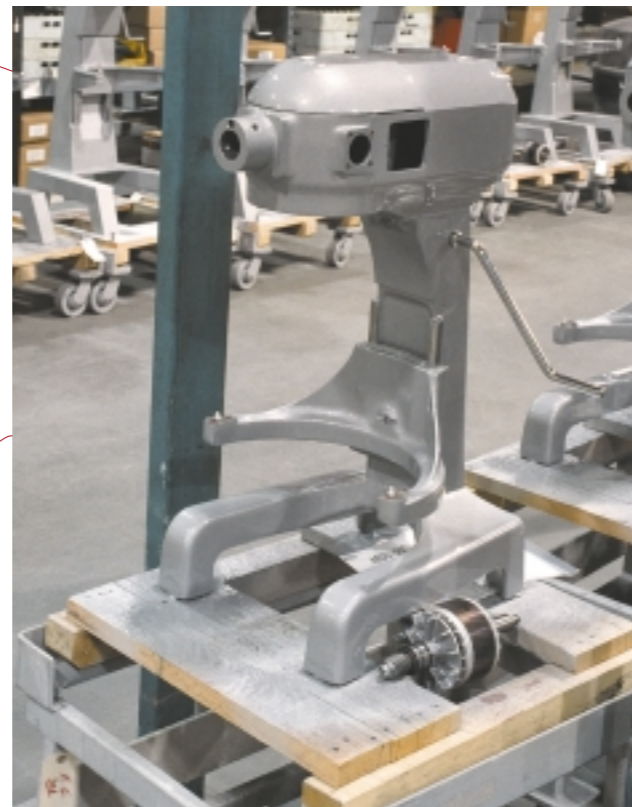
A mixer body is ready for the installation of the heavy-duty innards that have made Hobart the standard for the industry.
