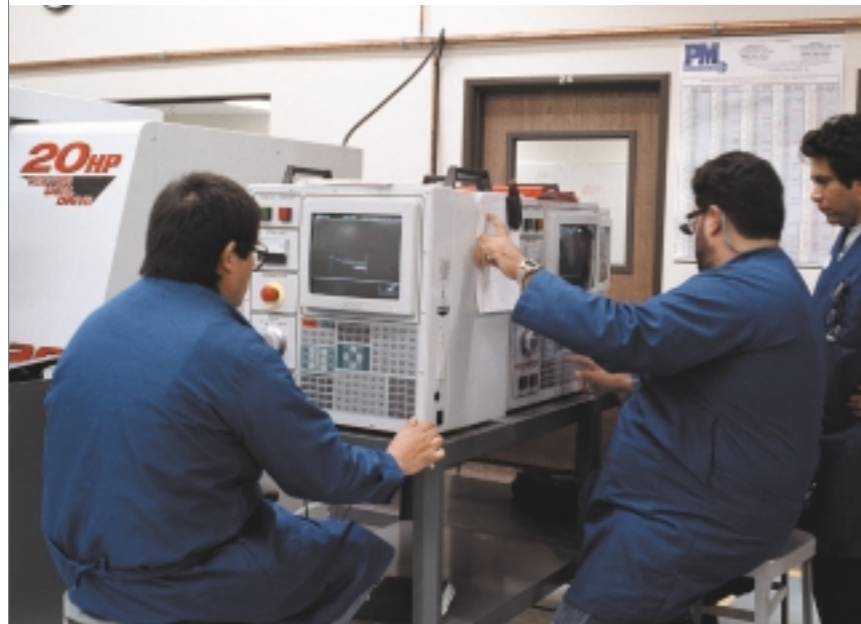
Haas control simulators provide more stations for training purposes, and allow students to learn machine operation independent of the machine. The VC-ATC has six total.
