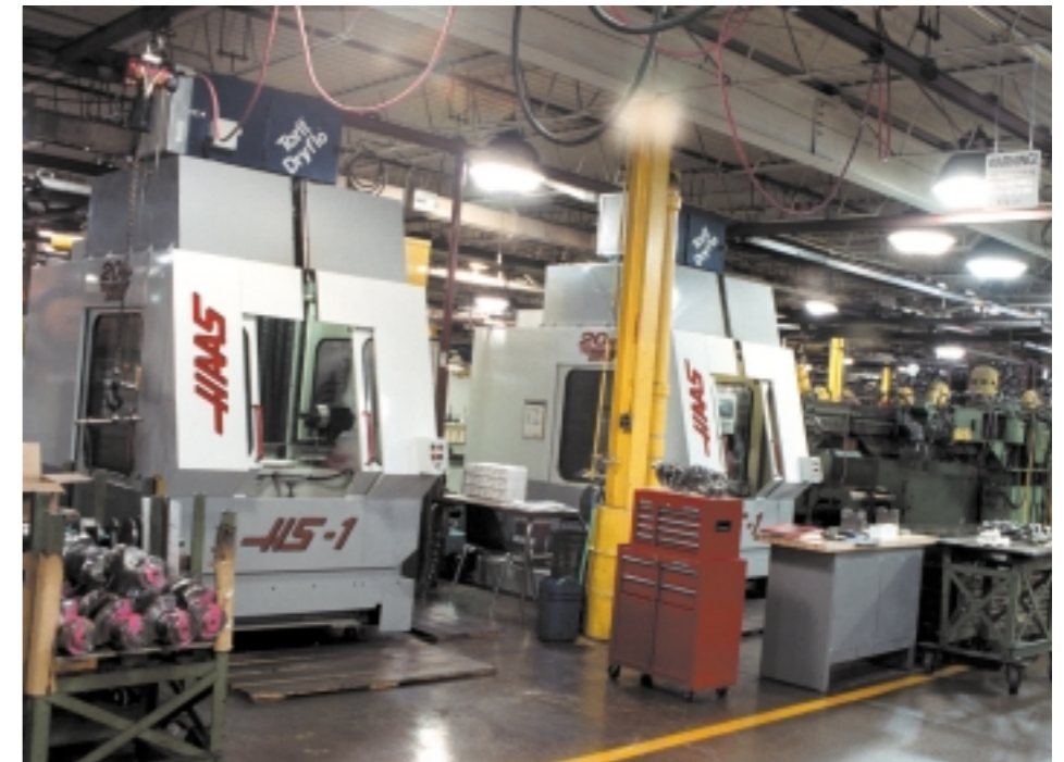
The HS-1R horizontals at Kellogg have been modified with a slot above the door to allow easy loading of weighty crankshafts using an overhead hoist.
