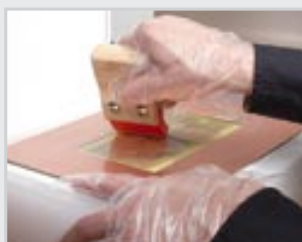
Using the squeegee to apply the conductor
