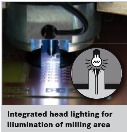
42,000 rpm high-performance spindle motor
