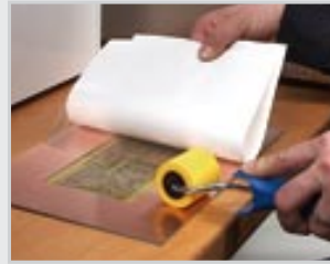
Applying the protective film
