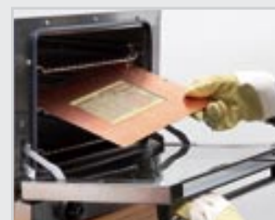
Curing the polymer in a hot-air oven
