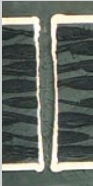
Conventional through-hole plating method (bone effect)
